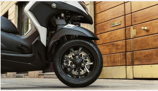
**Large diameter disc brakes with ABS**
